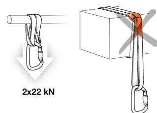
**Tested tensile strength**
