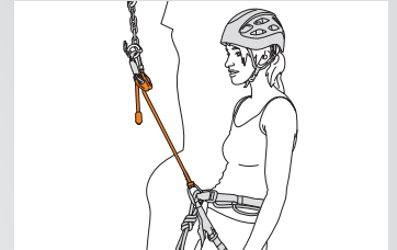
Adjustable and compact single lanyard for tethering to the anchor when climbing and mountaineering.
